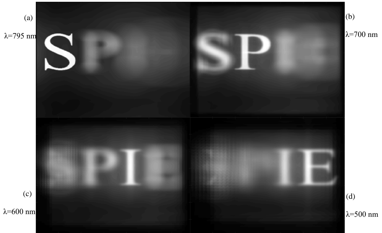
Figure 23. Hyperspectral image refocused with the DR algorithm at a) 795 nm, b) 700 nm, c) 600 nm, and d) 500 nm. The image contrast was adjusted to keep the image brightness comparable between images. The DR algorithm is able to refocus very well near design to differentiate wavelengths, however, as we get farther from design, that ability to differentiate wavelengths well disappears.
